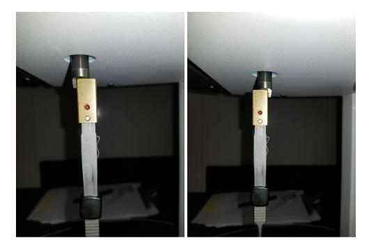
When tweezers move up, they will get caught either in the round opening in the bottom of the chamber or in the square opening on the top of it
