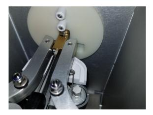
Vitrobot will lock down. If this ever happens, **do not** power cycle, since you can damage the motors by running them into a hard limit. Slowly step away from the instrument, put away your samples and tools and call for help.
